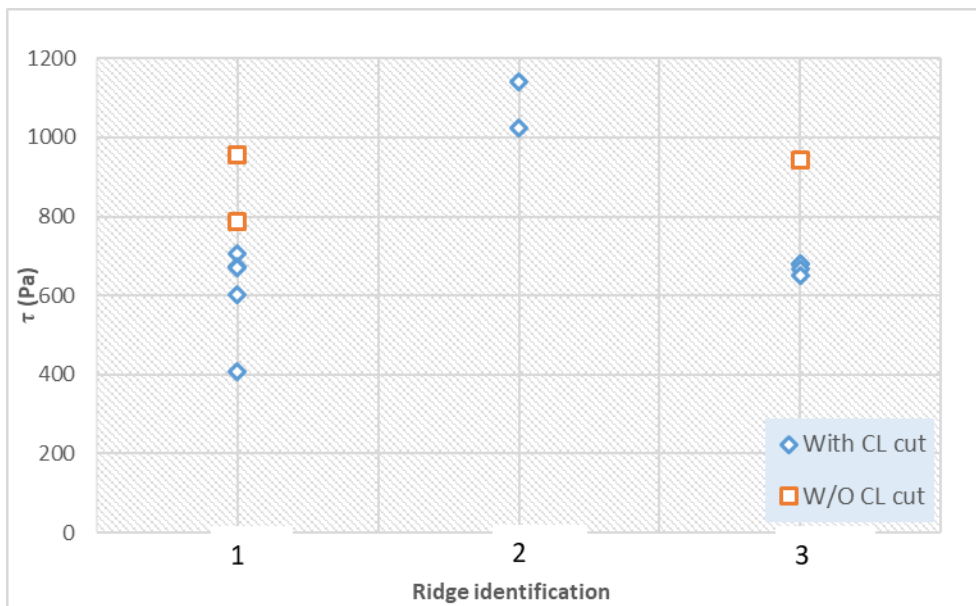
Figure 6. Shear strength of ice rubble determined from punch tests in three different consolidated ridges.
