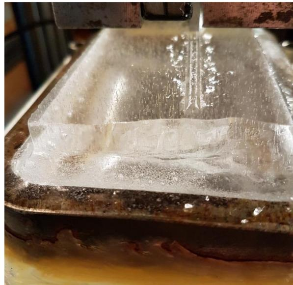
Figure 2. Blade track left following a number of gliding tests. Note that the vertical load is borne on the symmetric contacting portions of the blade’s edges. The thin white wispy material is frozen extruded slurry (discussed below).
