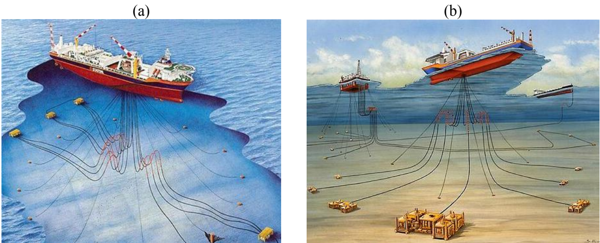
Figure 2. a) Development of the Norne field, 315 m water depth, off Mid Norway. b) The Åsgard development in 350 m water depth. A FPSO unit for the oil development, a semi submersible unit for the gas development and a storage unit for stable condensate (Gudmestad and Løset, 2006).
