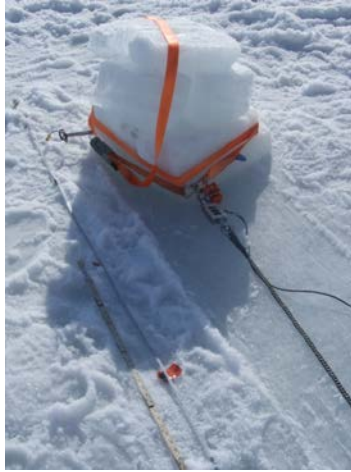
Figure 6. Test arrangement to study the influence of the normal load on friction.
