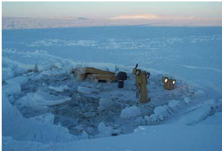
Figure 2. Breakthrough of a D10 Caterpillar tractor following a circumferential crack pattern. (Best practice for building and working safely on ice cover in Alberta, 2009)
