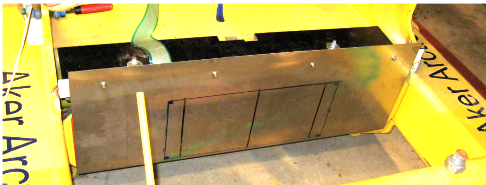
Figure 3. The tactile sensor protection plate. The plotted rectangle is the true location of the sensing area. The three vertical lines are the locations of stiffeners and give guidance to their positions in Fig. 5 and 7.
