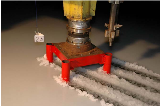
Channels formed during the structure passage through the ice ( L/D=6.0 ; \alpha=30^\circ )
