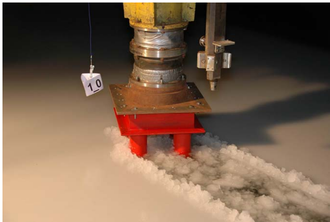
Channels formed during the structure passage through the ice ( L/D=2.5 ; \alpha=30^\circ )
