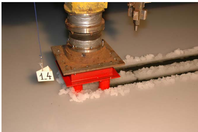
Channels formed during the structure passage through the ice ( L/D=2.5 ; \alpha=0^\circ )
