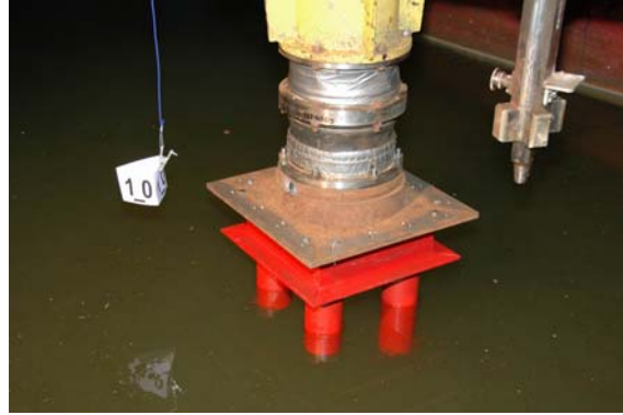
Figure 5. Four-leg structure model fixed through dynamometer to towing carriage and placed into the water before the tests
