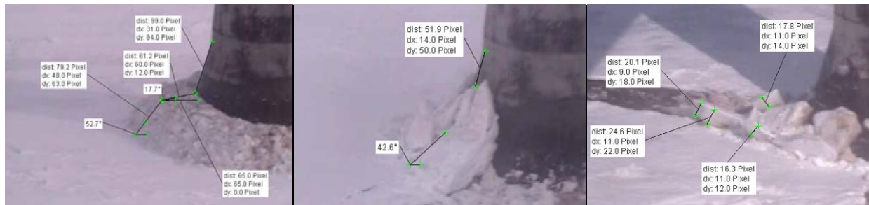
Figure 1: Typical example of image analysis for the measurements of rubble pile geometry (left), ride up (mid) and ice thickness (right)
