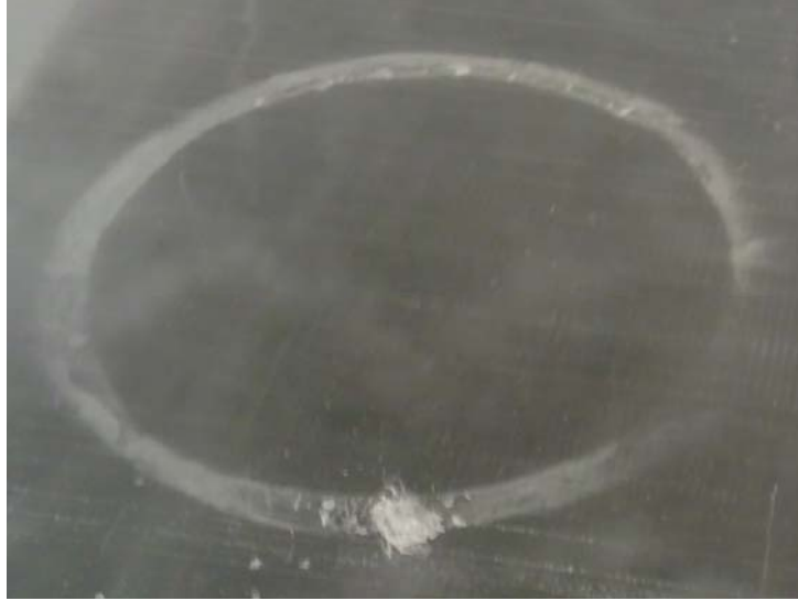
Fig. 8. Photo on the ice-ice contact where sintering is shown as a white spot.
