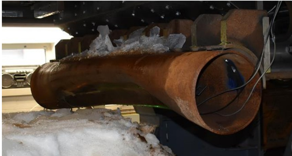
Figure 9. Schedule 40 pipe, post-test image showing deformed pipe
