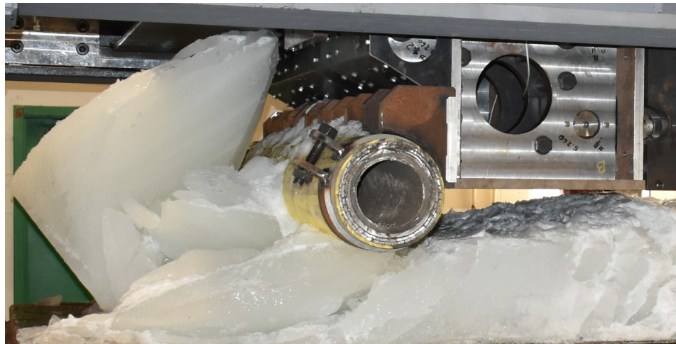
Figure 8. Flexible flowline, pre-test state (upper image), post-test (lower image).
