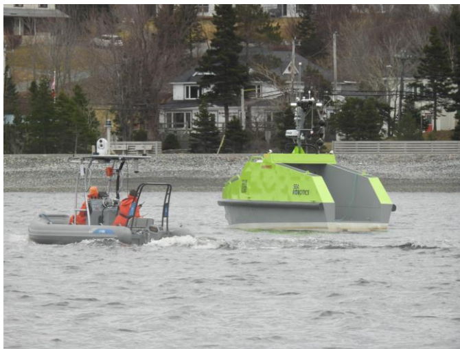
Figure 10. Two vessels (NRC-OCRE Acadia, left, and MI ASV, right) independently sensing each other and surrounding environment from different perspectives
