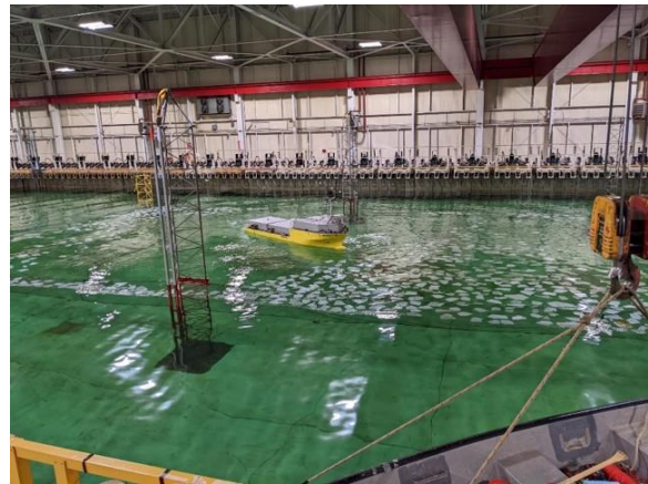
Figure 3. Model vessel traverses medium sea state with buoys (left) and plastic ice (right)
