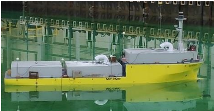
Figure 2. Model as-instrumented during basin trials
