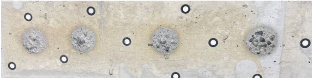
Figure 2: Abraded Sample Using Sandblasting Technique.
