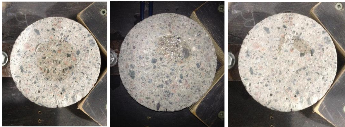
Figure 6. Darker grey “shadows” from ice bond with concrete, visible in most post-test imagery. (left) This example appeared to have near-perfect contact, with a shadow area covering 89% of the nominal contact area. In addition, there was some cohesive failure through the ice, with some ice remaining on the sample, visible in the upper left of the grey area. (middle) This sample had contact over approximately 44% of the nominal area, with ice remaining on the concrete for almost all of that area, visible as a shiny surface in this image. (right) This sample had coverage over only 20% of the nominal contact area, however it did also show cohesive failure through the ice where that bond occurred.
