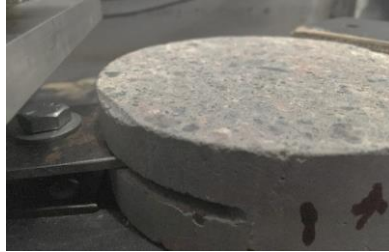
Figure 2. Concrete sample as prepared for testing and loaded into test apparatus.
