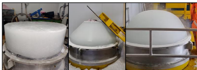
Figure 3. Ice cylinder before shaping (left). Ice cone being shaped (centre). Hemispherical ice cap being shaped by hand (right).
