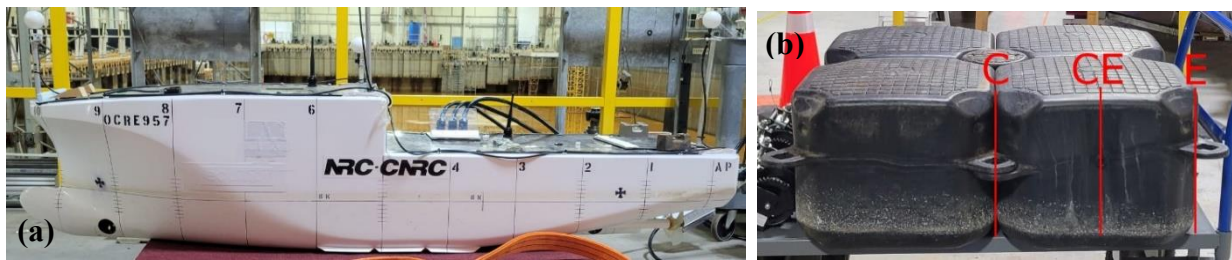
Figure 2: (a) The PSV model, (b) floating dock with position of impact marked.
