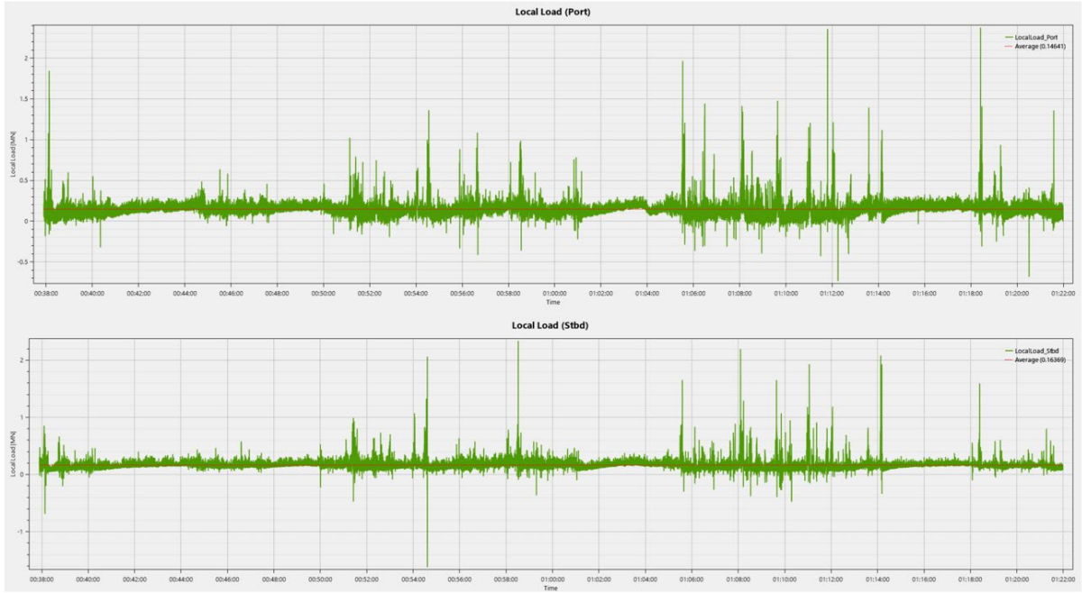
Figure 3. Time-Series of Measured Local Ice Loads (Port & Starboard)
