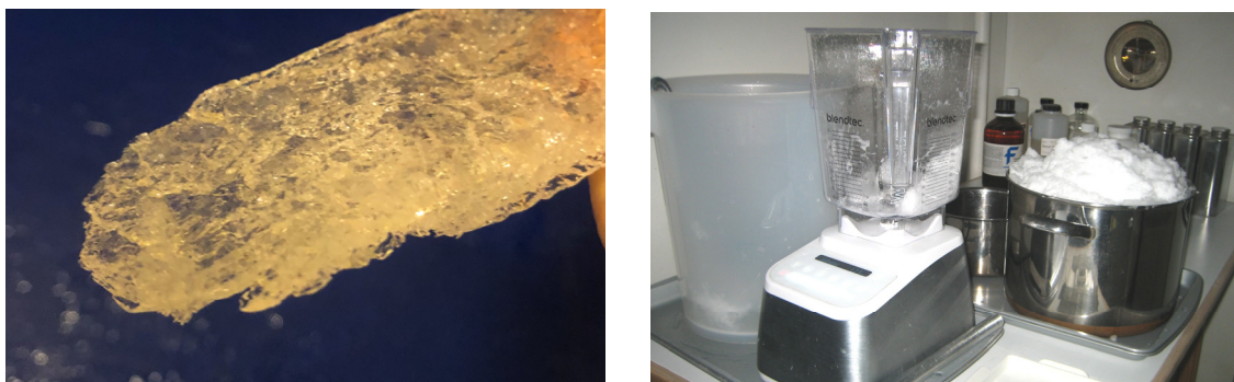
Figure 10. At left, example of the horizontal laminar structure and fracture pattern of a 'first ice' cantilever beam loaded to failure. At right, breaking up and grinding of the 'first ice' in the container at left with a blender (Designer 725 model by Blendtec) to produce fine grain slush at right. Short-lived foaming occurs even with low suds detergent.
