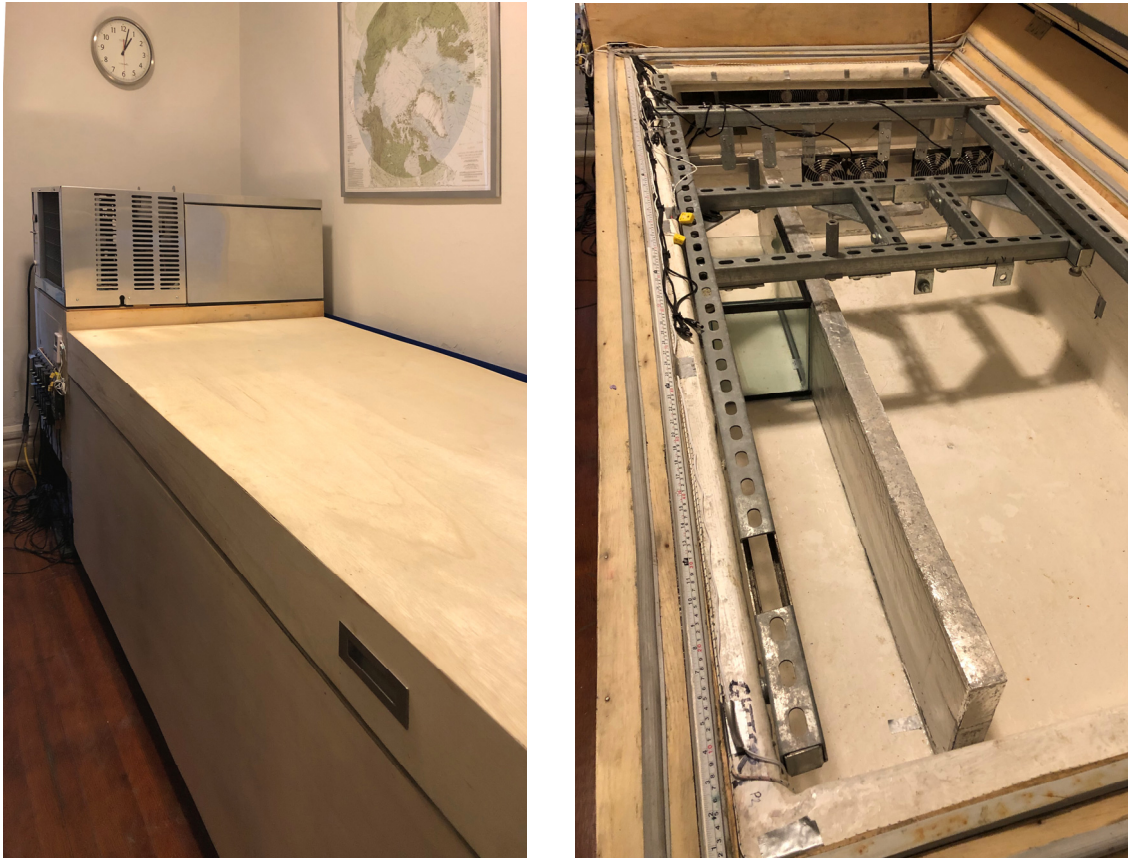
Figure 1. At left, the small ice towing tank with closed basin lid in foreground and packaged freezer unit at rear (For over-clad insulation added in 2024 and not shown, see drawings). At right, the fiberglass lined basin is visible with set up for an ice floe melt rate test.
