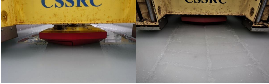
Figure 4. Level ice tests and pre-sawn ice tests
