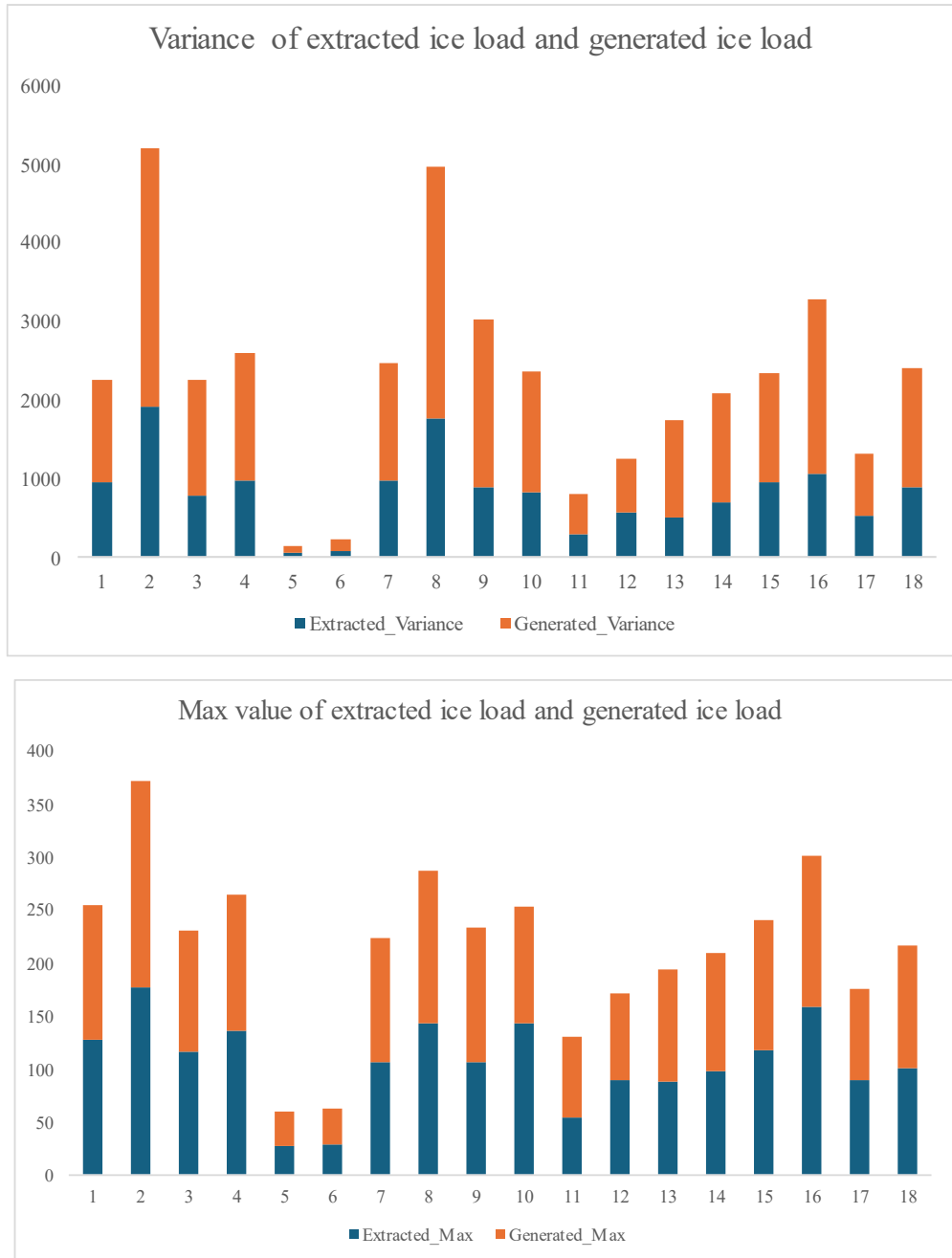
Figure 5. Statistical comparison of generated ice load fluctuation components and extracted ice load fluctuation components: a) variance; b) maximum value
