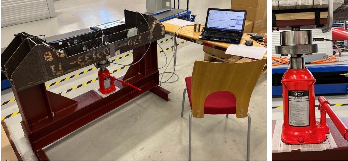
Figure 3. Test rig (left), consisting of frame, test piece, loading device (shown in more detail on right) and measurement setup.
