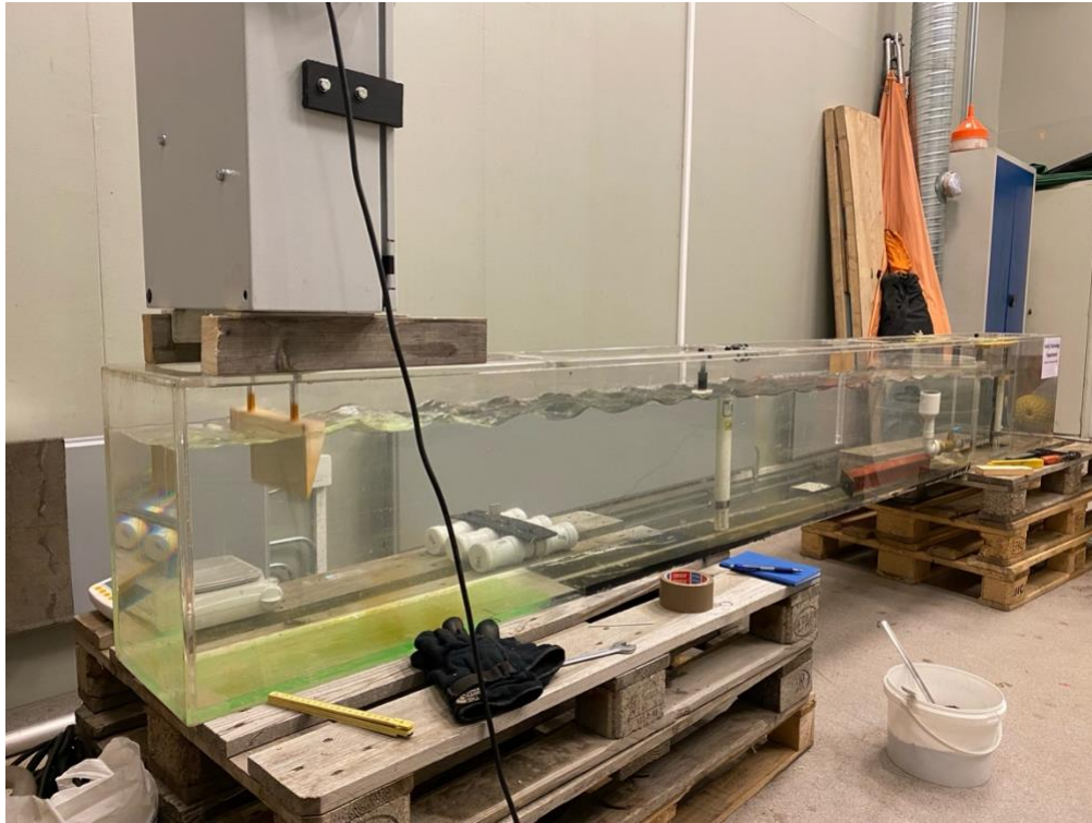
Figure 1. Flume with wave maker at UNIS.
