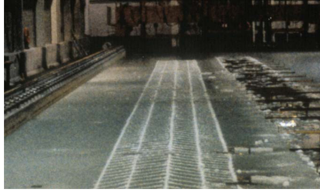
Figure 3. Cutting pattern of pre-sawn ice ( ITTC, 2017 )
