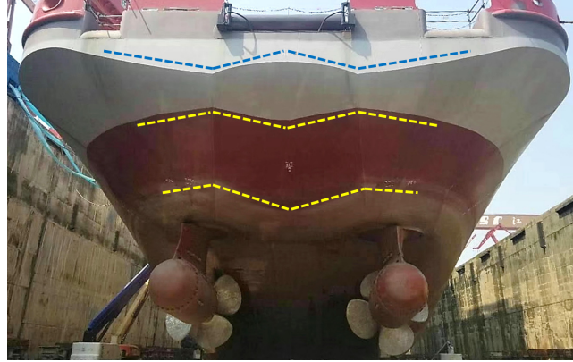
Figure 4. Stern of the Chinese polar research vessel Xue Long 2 . Dashed lines illustrate the W-shaped profile from either the horizontal or transversal section.
