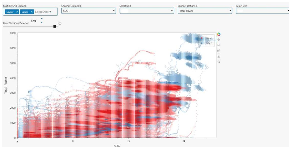
Figure 6. Performance Scatter plot for two ships
