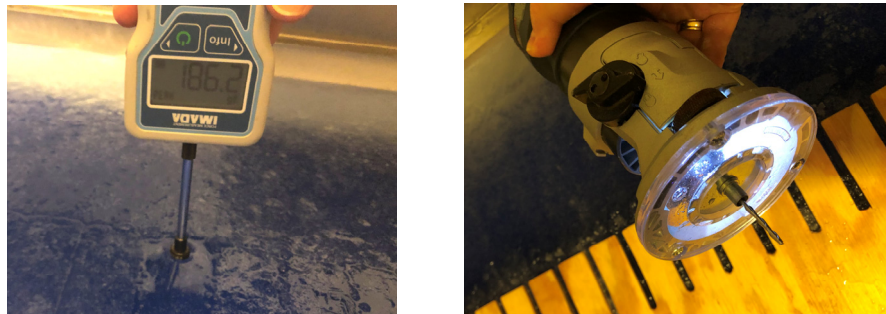
Figure 10. At left, measurement of flexural strength with cantilever beams using a DST-1A force gauge. At right, cutting of cantilever beams in an untempered ice sheet with plywood guide. (A wider diameter bit to reduce stress risers at cantilever roots is being developed.)
