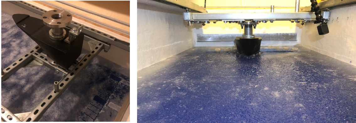
Figure 1. At left, preparing the icebreaking bow for installation on the towing carriage during in-situ testing of cantilever beams. At right, the 10 kPa target has been reached and the bow is ready for testing. 16 Jun. 2024.
