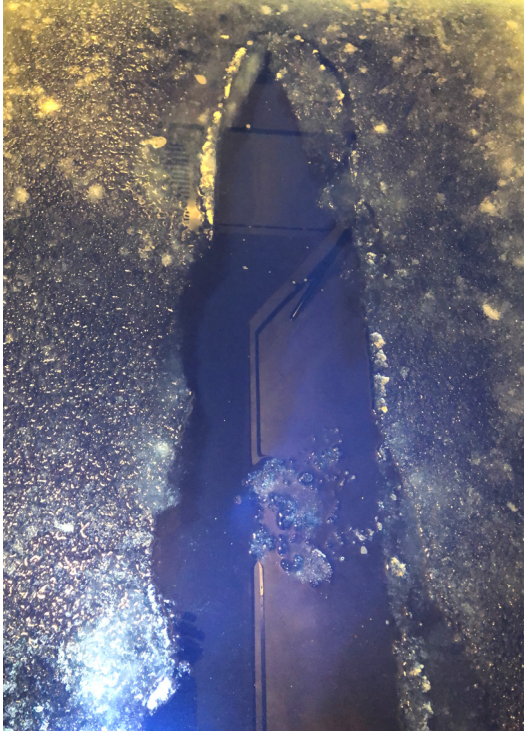
Figure 3. At left, an overhead view of test results for the icebreaking bow. Partially submerged crescent shaped fragments are visible with most having been cleared when retracting the model. At right, the undisturbed condition just after the test. There is often increased breakage adjacent to the in-situ beam test zone in the foreground. 16 Jun. 2024.
