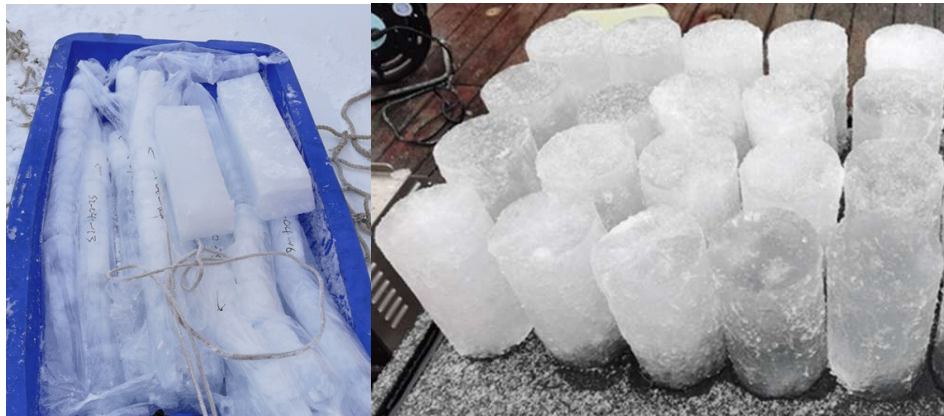
Fig.2 The collection and preparation of the sea ice samples
