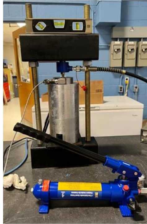
Figure 1 – (a) Conceptual design of the pressure melting observation apparatus; (b) Apparatus in loading frame with hydraulic hand pump.
