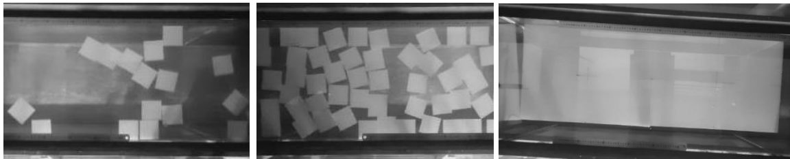
Figure 2. Laboratory model of ice, shown in the images from left to right for low concentration conditions, high concentration conditions, and an ice cover
