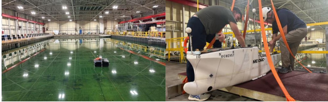
Figure 3. Ocean Engineering Basin and PSV model before testing
