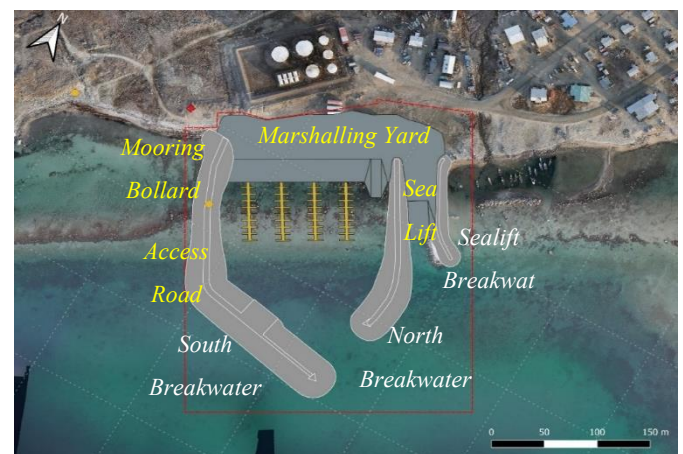
Figure 1. Harbour Layout, developed by CBCL
