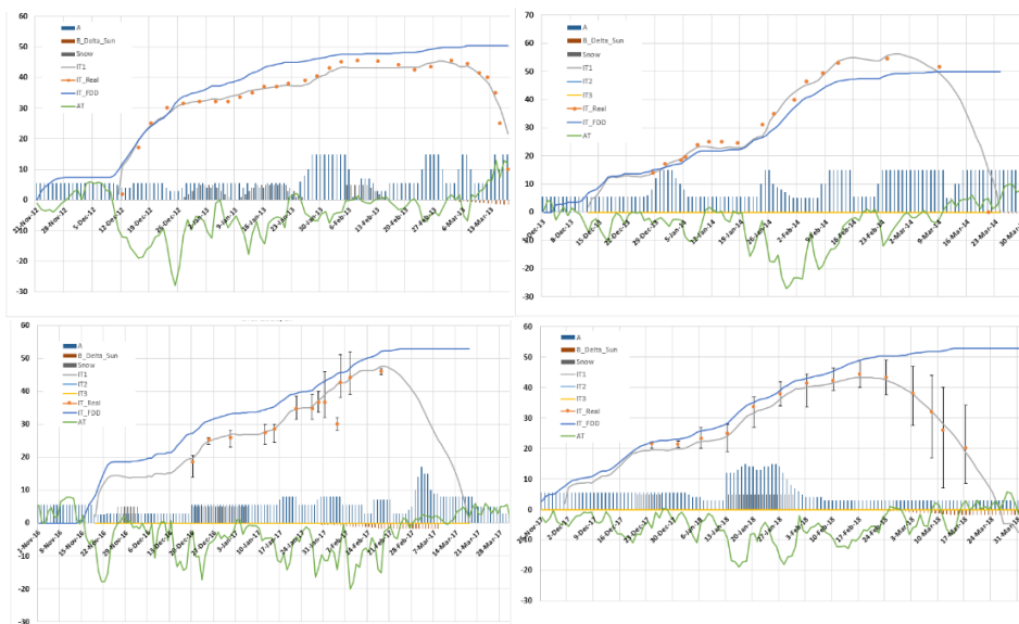
Figure 2 Examples of thermal model performance verification with physical measurements data and comparison with model considering only negative degree days.
