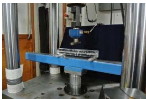
Figure 1 Test set-up of the simple beam test
