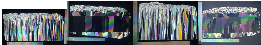
Figure 3 Through thickness vertical thin sections of ice blocks: (a) Cooler1 showing the S2 structure, (b) Cooler2 showing the T3/S1 structure, (c) Cooler3 showing the S2 structure, and (d) Cooler4 showing the T3/S1 structure. (Samples a-d are shown from left to right).
