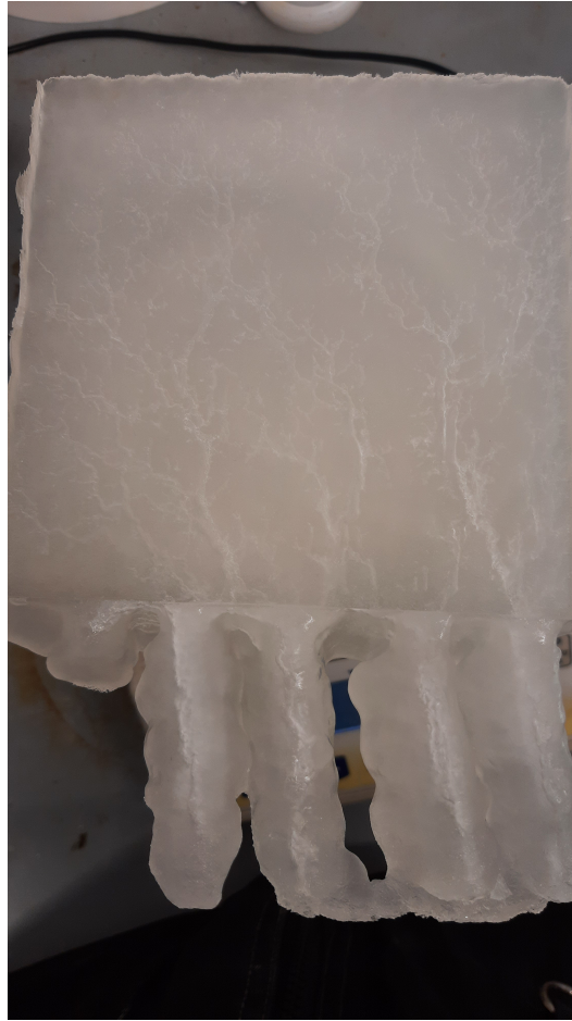
Figure 3: A sample after the adhesion test. Icicles formed on the lower end of the sample, brine channels are visible with eye and camera on the former interface. Small ice walls on the side of the sample show that icing around the edges occurred.
