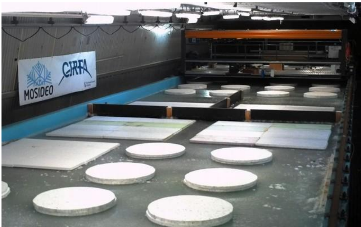
Figure 4. Surface insulation to create an under-ice profile.
