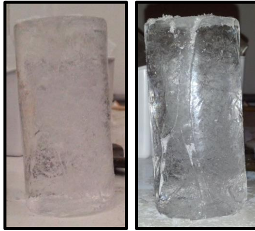
Figure 2. Two inch by four inch cylindrical ice samples
