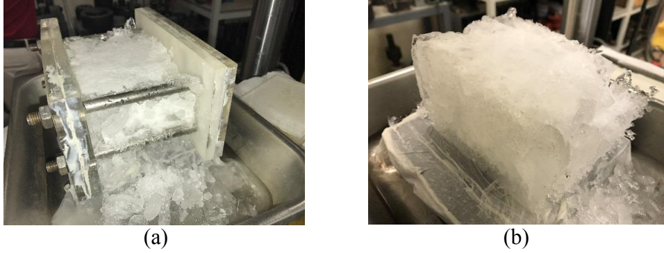
Figure 17: (a) Crushed ice under lateral confinement and (b) view of granular ice fragments with confinement platens removed.
