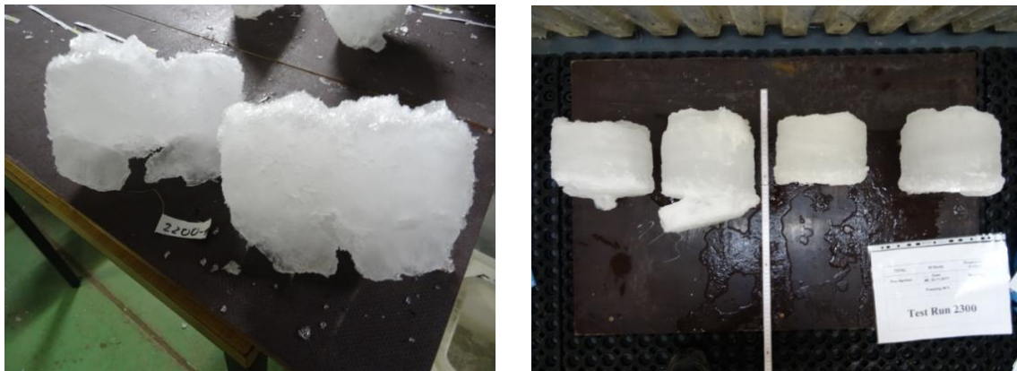
Figure 3-2. Examples of cores taken after 24hrs (left image) and 48hrs (right image). Brash ice pieces frozen on the bottom of the samples can be clearly observed with variation in lower ice surface.
