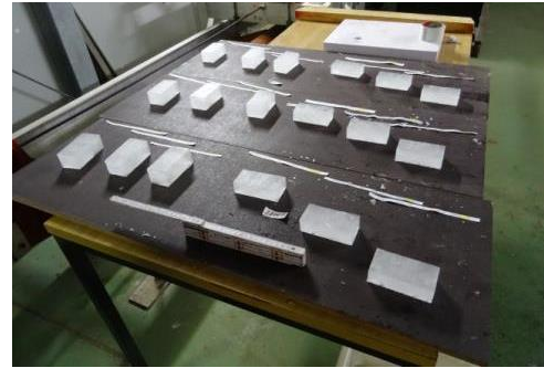
Figure 3-3. Illustration of cutting scheme for compressive strength (left image) and layout of the samples for compressive strength testing taken from one core (vertical samples on the left side of the image and horizontal samples on the right side of the image).
