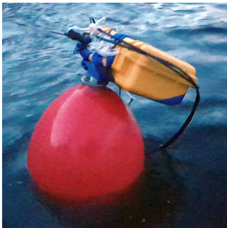
Figure 3. Direct deployment of logger and temperature cable from a boating buoy.
