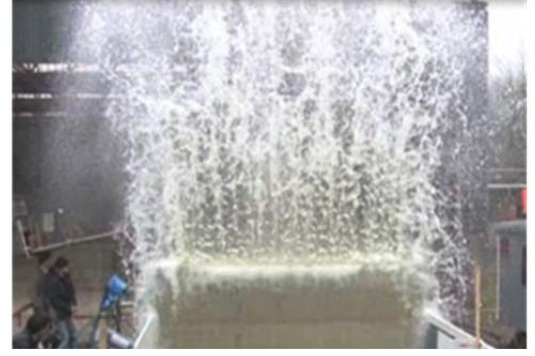
Figure 9: Run-up jet from a sloshing experiment breaking up (Bogaert, 2010) showing streaks formed.
