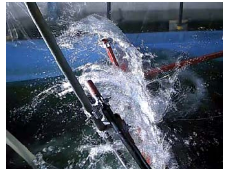
Figure 4: Typical side view of a jet formed at a backward (-15°) inclined wall after run-up.
