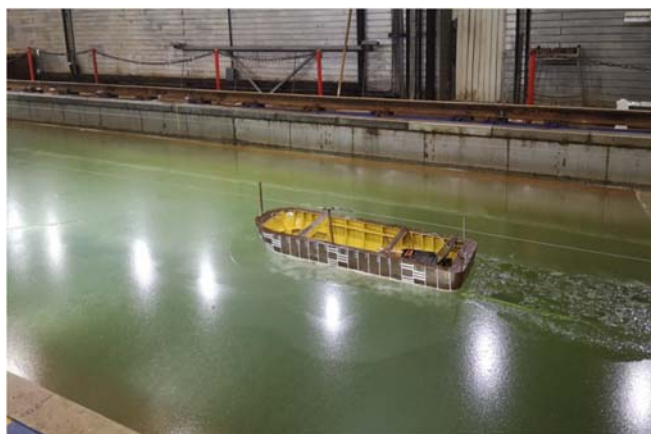
Figure 2. Trials of the IRSPP model in level ice in the AARI ice tank
