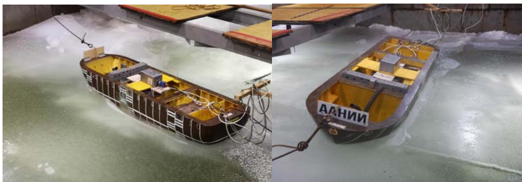
Figure 3. Trials of the IRSPP model at compression in ice in the AARI ice tank
