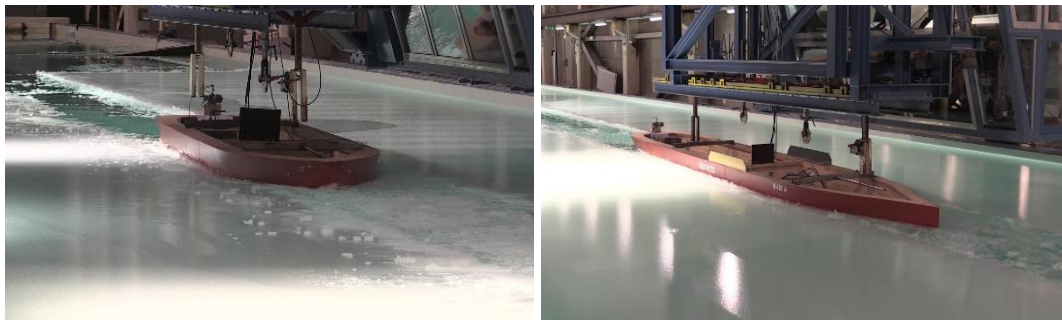
Figure 14. Attempt to break out from channel with Reference ship (left) and EEDI bow (right)
