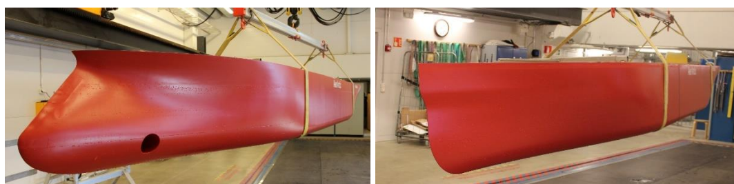
Figure 6. Models of the reference ship (left) and EEDI hull form (right)
