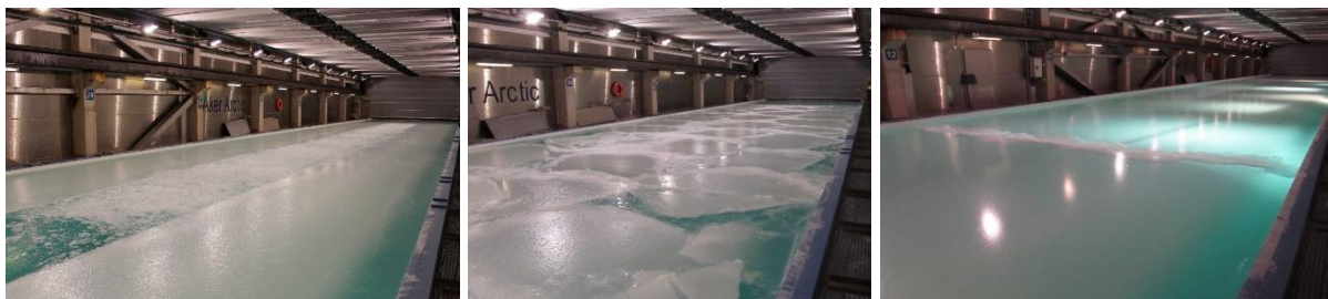
Figure 7. Ice conditions in model tests: brash ice channel (left), pack ice (mid), triangular ridge in level ice field (right)
