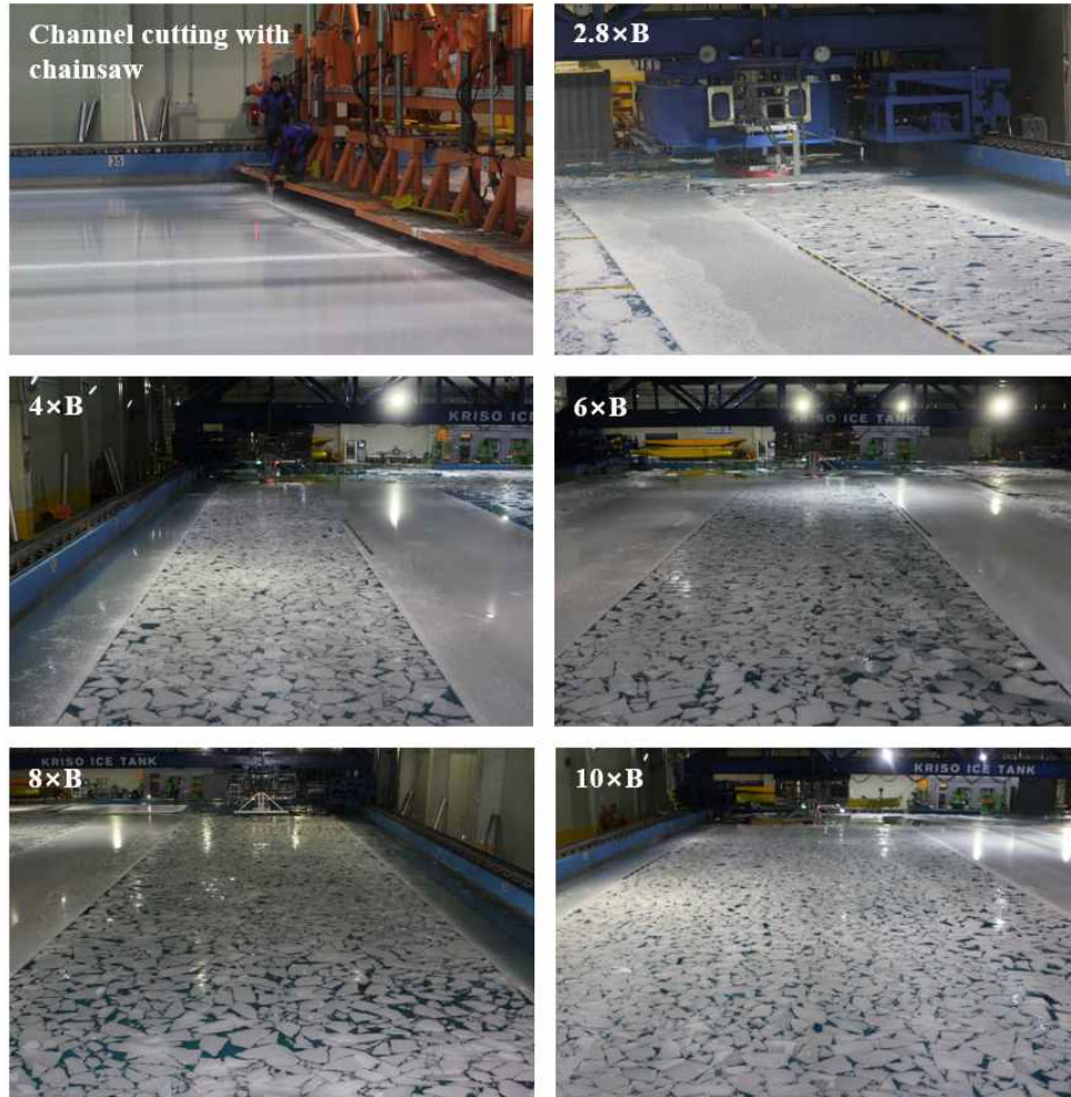
Figure 3. Various channel width conditions at 80% ice concentration
