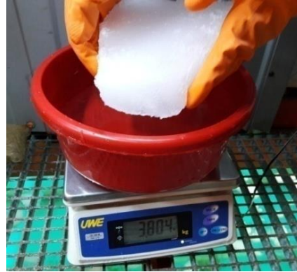
Figure 6. Measuring the rate of water draining from the ice specimen
