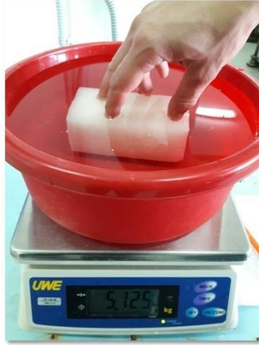
Figure 2. Paraffin specimen submersion performed by hand
