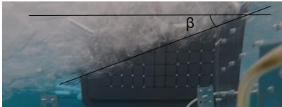
Figure 6. Angle of repose below water
