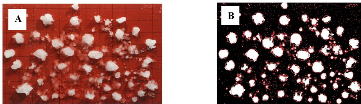
Figure 4 A: Photograph of brash ice. B: The brash ice after processing in Matlab.
