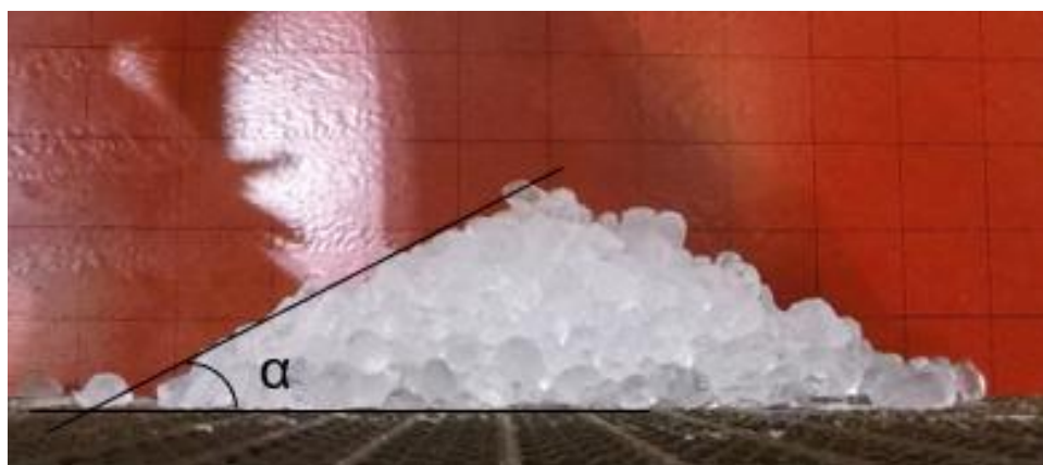
Figure 7. Angle of repose above water
