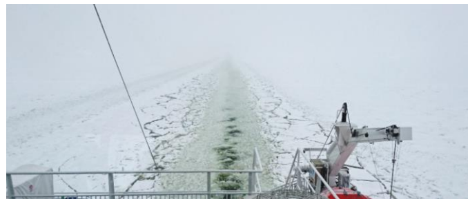
Figure 2. Newly broken brash ice channel
