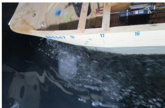
Figure 7. Towed self-propulsion tests with running ahead and astern
