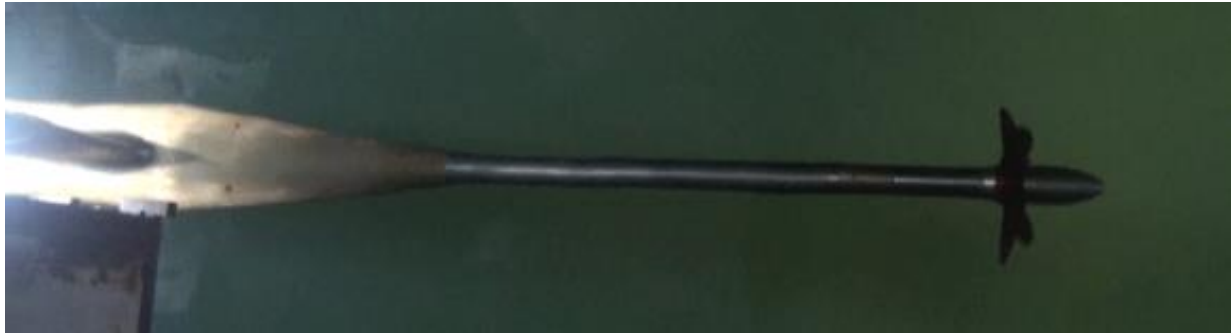
Figure 6. Propeller open water tests
