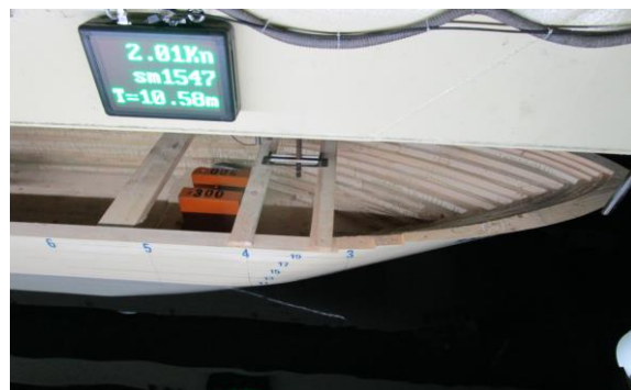
Figure 7. Towed self-propulsion tests with running ahead and astern
