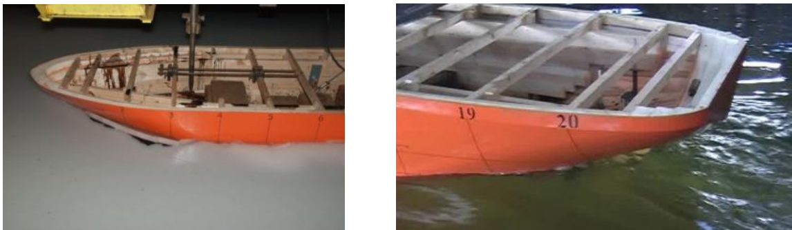
Figure 3. Model tests in ice and open water at KRYLOV
