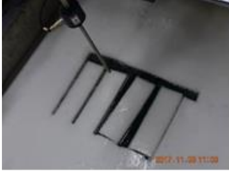
Figure 6. Flexural strength / elastic modulus measurements on ice sheet
