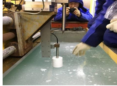
Figure 6. Flexural strength / elastic modulus measurements on ice sheet
