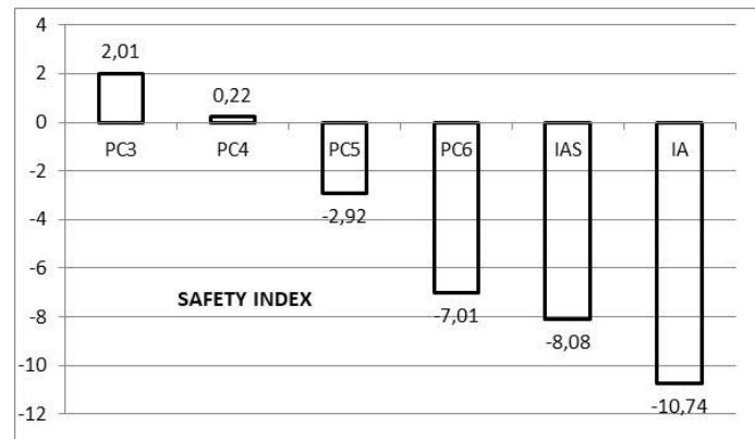
Fig.6. Safety indices of the bow frames of MT Uikku (Kurmiste, 2016)
