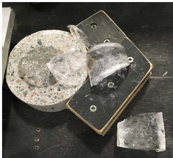
Figure 8 Example of catastrophic cohesive failure during a preliminary test.
