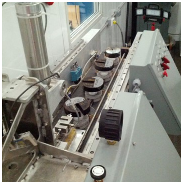
Figure 6 Samples with 2.25 kg weights, after 24 hours of loading, ready for testing. Weights were removed immediately prior to the start of the tests.
