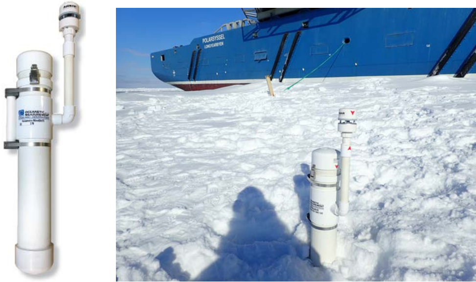
Figure 2. Left panel. Ice tracker Oceanetic Measurement equipped with anemometer. Right panel. Ice tracker deployed on the drifting flow on April 24, 2017.
