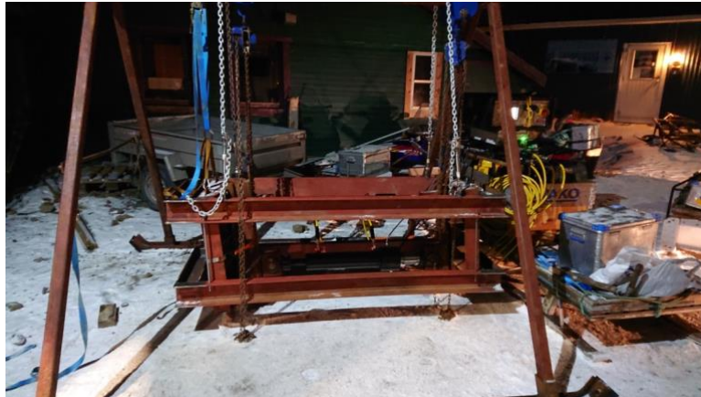
Figure 5. Steel frame for the calibration of the indentation rig. The rig is inside the frame.
