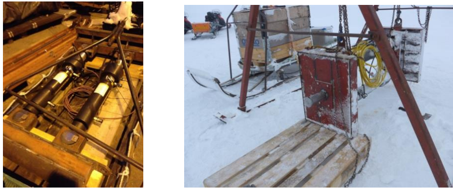
Figure 1. Hydraulic rig to conduct full-scale tests to measure ice strength. Left panel shows the indenter packed on sledges. Right panel shows an indenter mounted on an A-shaped frame with sledges.
