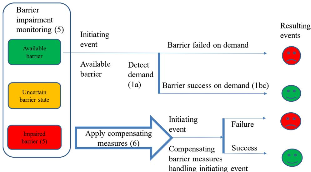
Figure 7. The box to the left indicates operational monitoring barrier states (availability/impairment). The upper event tree presents the normal barrier events (1abc). The blue arrow and lower event tree represents how the operator may decide to apply predefined compensating measures(6) in case of indicated barrier impairment(5).
