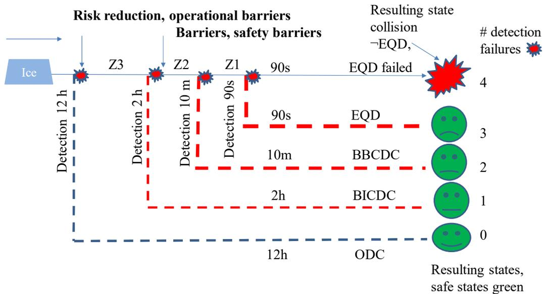
Figure 6. Barrier system event tree model with four simplified detection barrier branches leading to the defined four safe states (ODC, BICDC, BBCDC, EQD) for the BOP. Note that the specific alert actions and associated BOP actions are not included in the figure. The number of detection failures for the different resulting states are indicated in the right column.
