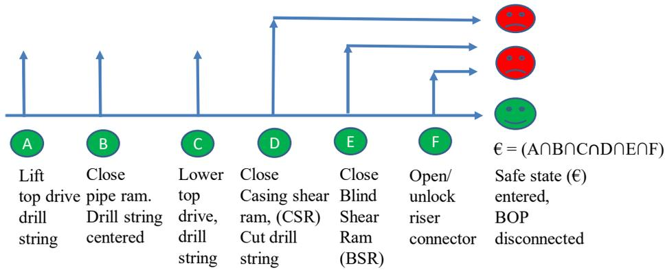
Figure 10. Illustration of detailed BOP actions in an event tree for the operator barrier panel.
