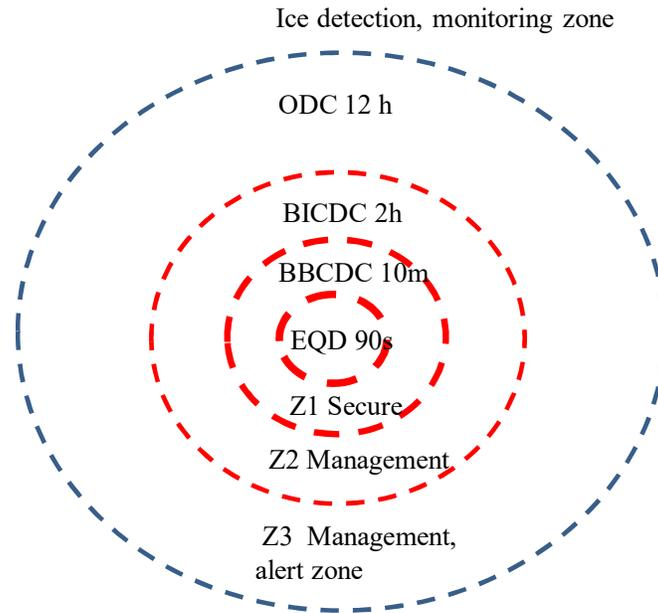
Figure 5. Four IM zone definitions (ISO 35104-2018) for the example Blow Out Preventer (BOP) case indicating required termination time for entering the defined safe states.
