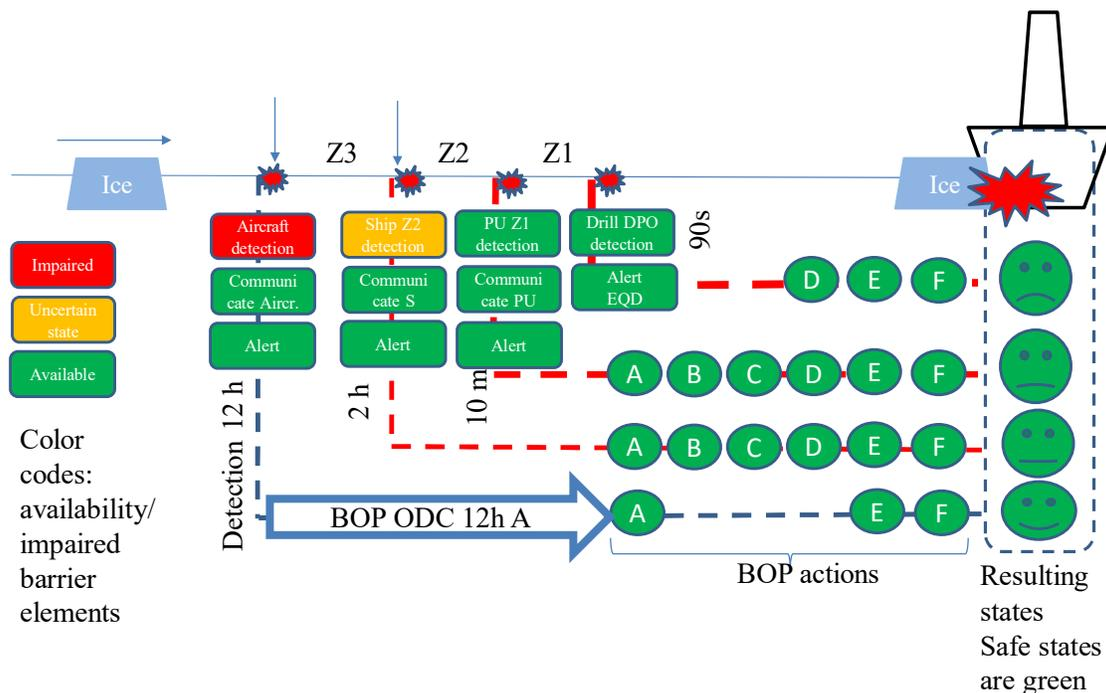
Figure 9. Operator barrier panel presented as an event tree with operating state of 4 barrier branches and color codes for the availability of the specific barrier elements. The impaired barrier elements are shown as Aircraft detection (red) and Ship Z2 detection (yellow). The available compensating measure is shown as a blue arrow for starting BOP action “A” which is to hoist/lift the drill pipe.
