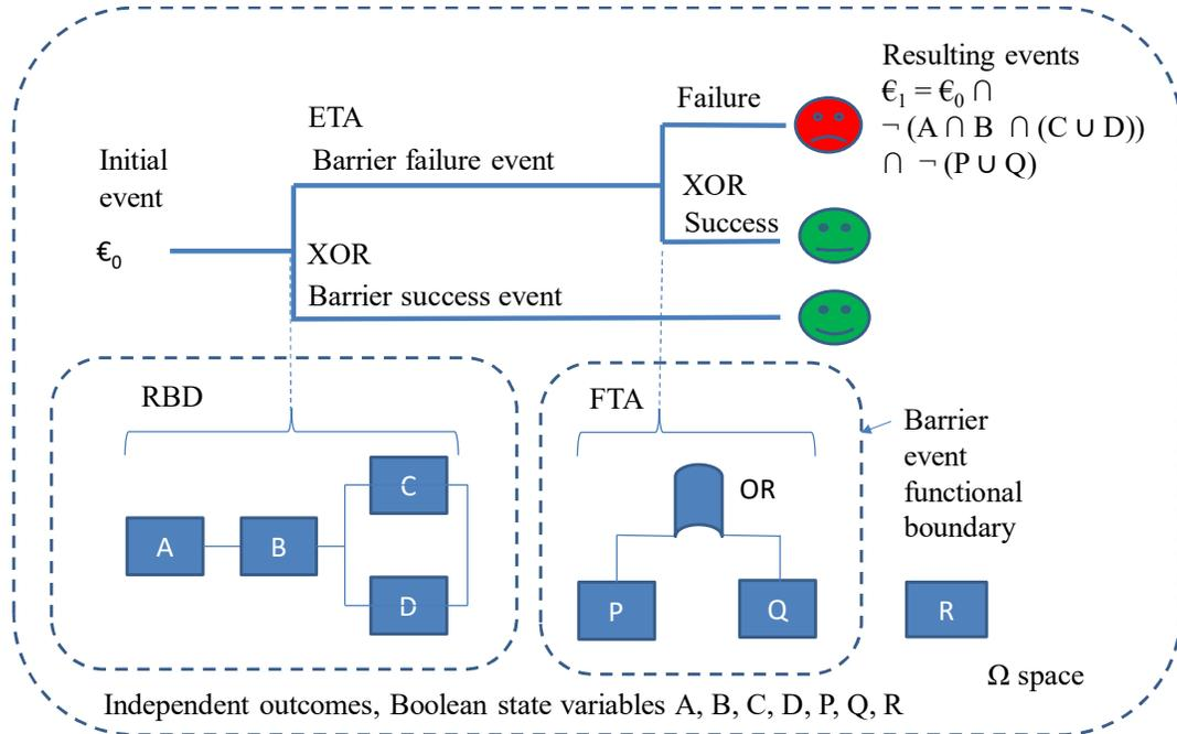
Figure 12. Measurable space with Boolean state variables (outcomes, A,B,C,...) enabling representation of barrier events ( $\epsilon_0$ : Initial event,  $\epsilon_1$ : Resulting event). Event tree (ETA), Reliability Block Diagram (RBD), and Fault Tree (FTA) are Boolean expressions with state variables and Boolean operators ( $\cap, \cup, \neg$ ) in a Sigma algebra/space.
