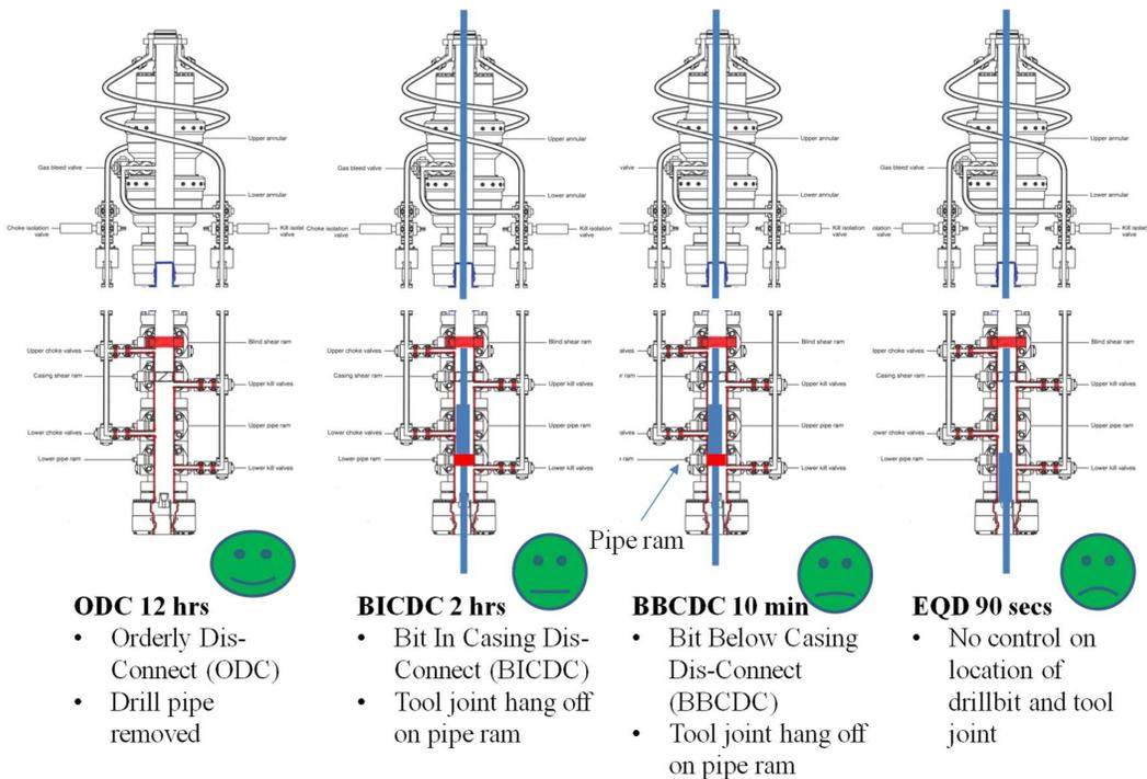
Figure 4. Four safe states (ODC, BICDC, BBCDC, EQD) for the example BOP case (Courtesy DNV GL, DNVGL-OS-E101: 2018).
