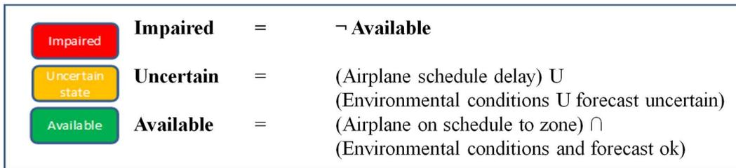
Figure 8. Principle for high-level specification of performance requirements for barrier panel presentation of status and availability color codes of barrier element Aircraft Z3 in Figure 9.
